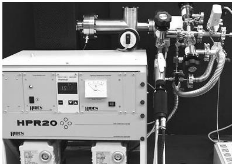
Fig. 5 The Hiden HPR20-QIC mass spectrometer with solid insertion probe
